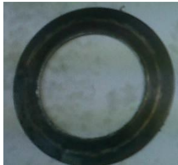
Bell/Thrust Washer that may be added
